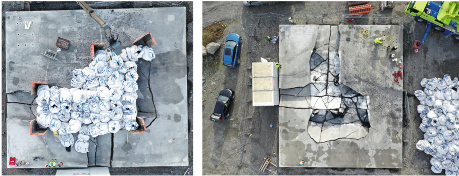
Fig. 11. Photo after failure – before and after removal of the loading bags.
