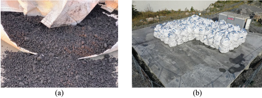
Fig. 4. Loaded slab: (a) loading material; and (b) placement of the loads on the slab.
