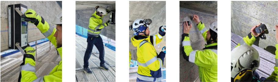
Fig. 5. Inspecting grouting conditions with MIRA and Impact Echo
