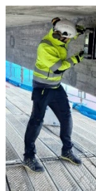
Fig. 5. Inspecting grouting conditions with MIRA and Impact Echo
