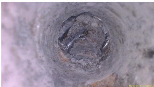
Figure 56 Opening 4N (left) and 6N (right) - Images of duct 33N with grout
