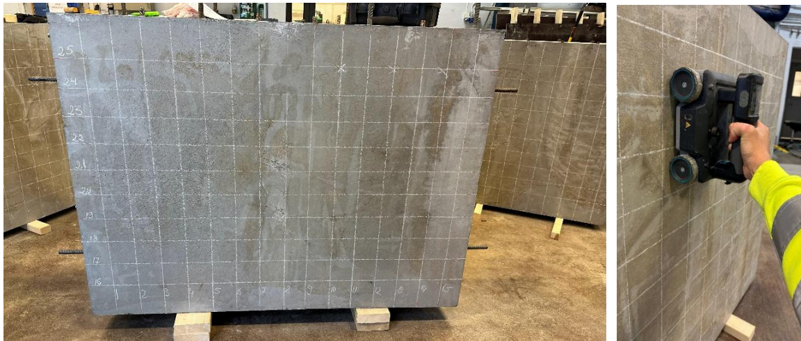
Figure 20 defined gridlines on the concrete surface and scanning along the scan lines
