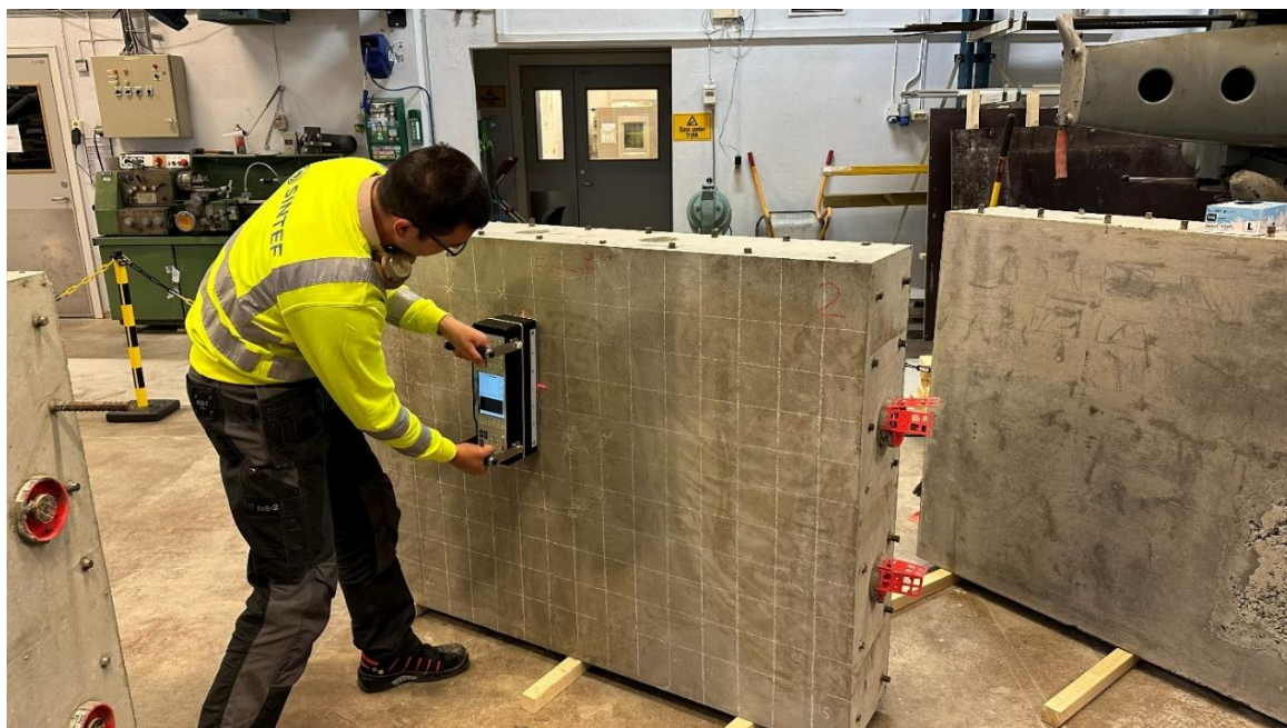
Figure 21 Ultrasound scanning, using MIRA A1040
