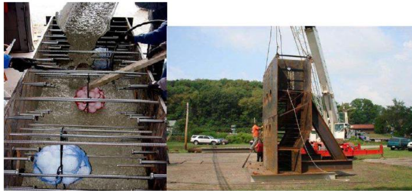
Figure 10 Fabrication of mock up specimens (from (Wiggenhauser et al., 2015))
