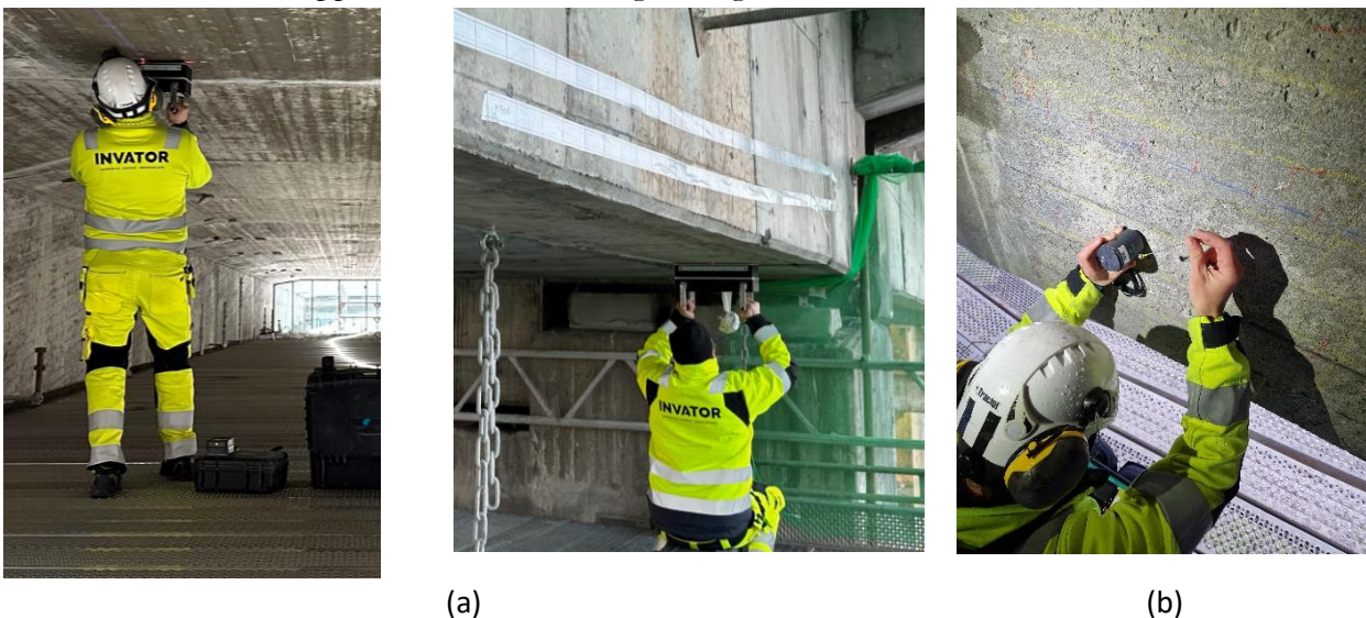
Figure 41 Field inspection of grouting conditions with: (a) MIRA ultrasonic array positioned on the concrete surface inside the box girder, capturing multi-channel I/Q data for coherence-based void detection, and (b) Impact Echo testing attempted for complementary resonance validation
